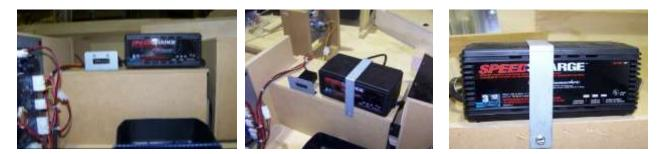
Install the battery cable as shown below. For easier access the battery is not secured – When moving the table the battery should be removed or secured to prevent damage. When the battery is removed – put the protective cover on the battery cable.
