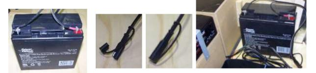
For the final step: connect the Battery Cable to the Charger cable using the single position safety connectors
