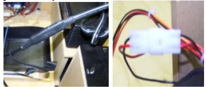
Connect the 2 pin Molex connector from the Charger to the Main Harness.
