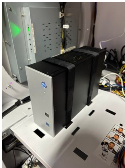
Front of computer, secured by industrial velcro straps. Ports are on back side.
