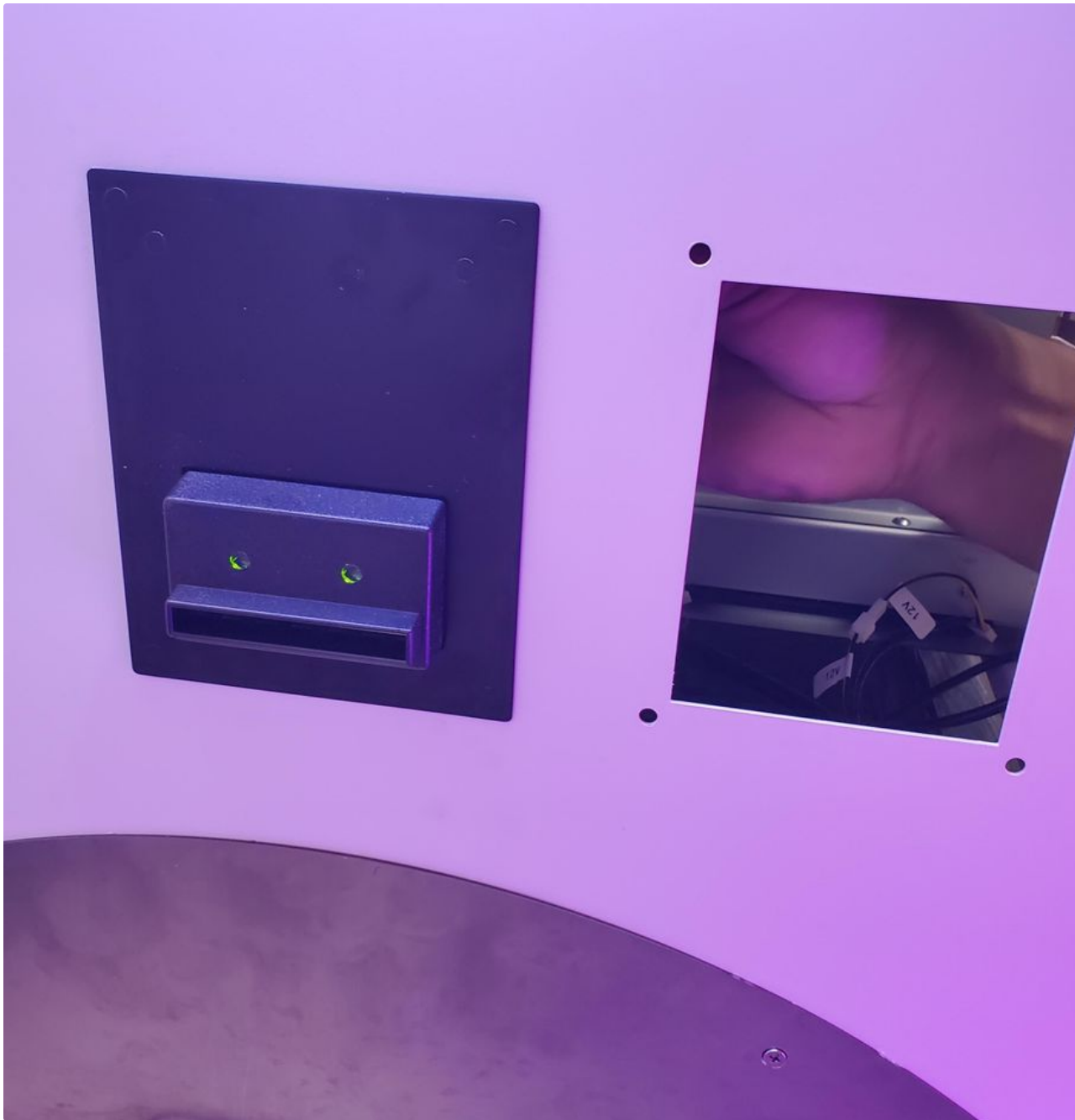
DBA installed from outside - upon wiring correctly, green lights on front of DBA should blink twice regularly
