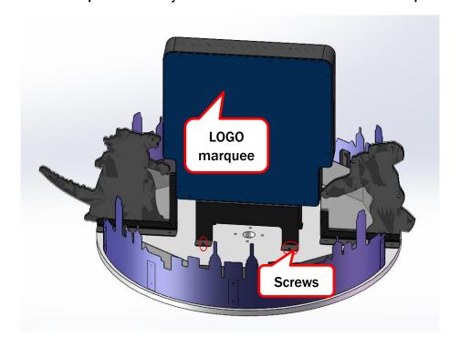
Step 3-1 Place Marquee assembly to the top of the loops assembly. Utilize screws to secure.
