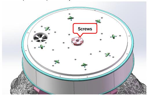
Step 2 Locate Marquee assembly. Loosen screws to remove LOGO marquee.
