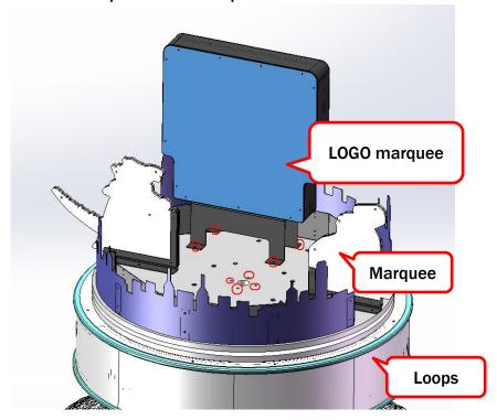
Step 4 Loosen 4 screws on the 4 positions.
