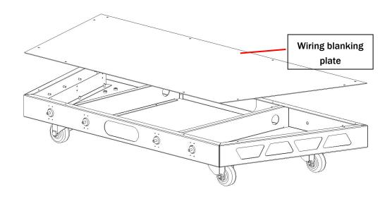
Step 4 Place Wiring box the the Cabinet bottom side. Through the cabinet connectors to the wiring box. Utilize screws to secure. Adjust the Wiring box leveller
