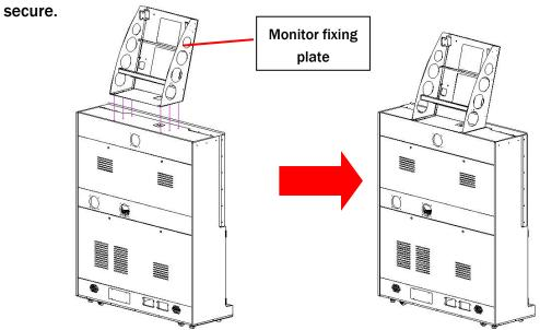
Step 2 Place Monitor to the fixing plate. Monitor connector through the square wiring hole to the back side. Utilize screws to secure.
