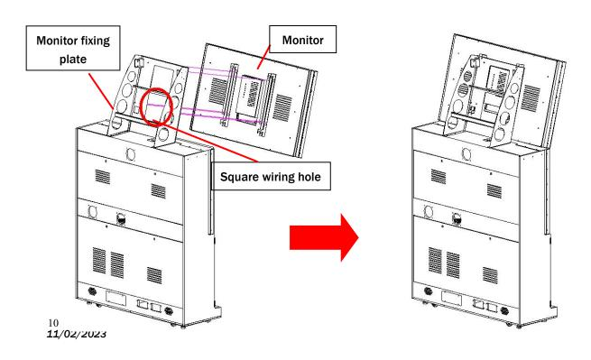
Step 3 Open Back upper door. Place Marquee to the top of the Monitor. Utilize screws to secure.
