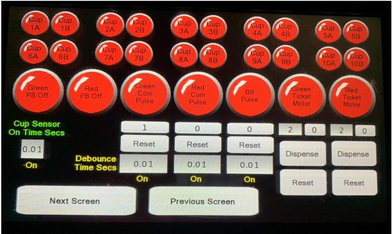
The pulse “On” time can be entered for the Green Coin, Red Coin and Bill Pulse. The fastest pulse time that you can enter is 0.01 seconds. The pulse “Off” time does not need to be entered.
