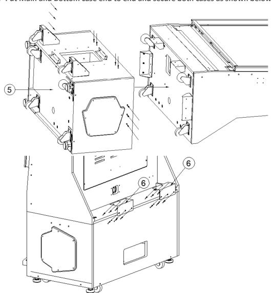
C. Assemble the brackets as shown in the picture.
